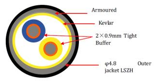
This is armored fiber optic patch cord with 2 fibers, which is designed ideal for CPRI cabling system.
